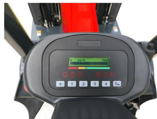
ZAPI dashboard displays failure codes
